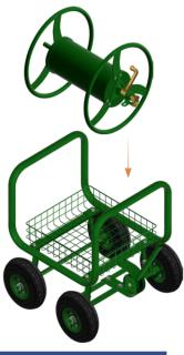
Place Assembled Hose Drum (F) onto the Frame.
