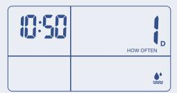
Rain sensor is triggered state, and the icon flashes every 0.5 and the flashes every 0.5 seconds.
