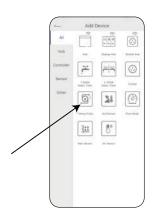
Hold the SET button on the side of the pump until the red LED light quickly blinking. Then select "Next" on the APP to start searching device.
