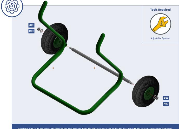
Insert the Axle (2) to the Frame (1) through the Axle Mounts. Slide the Wheels on to each end of the Axle (2) with the Valve Stems Facing Outwards.
