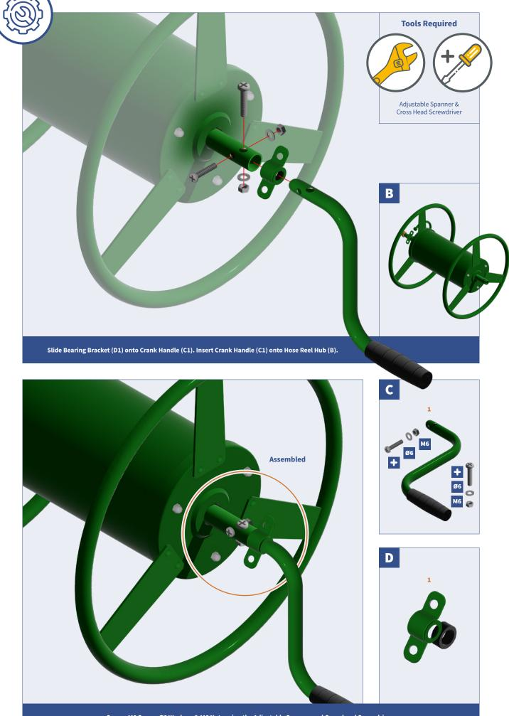
Secure M6 Srews, Ø6 Washers & M6 Nuts using the Adjustable Spanner and Cross head Screwdriver.
