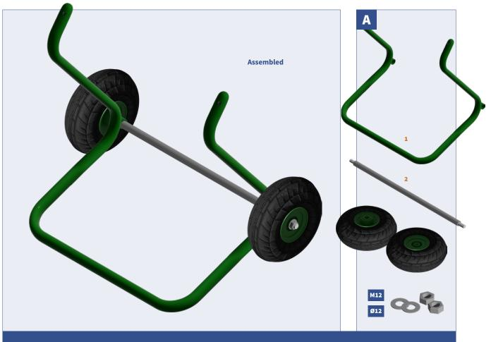
Attach Wheels using Large Ø12 Washers and Large M12 Nuts. Secure using a Spanner.
